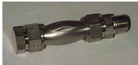
Figure 3.2.1 - 2, Burst Test Configuration
