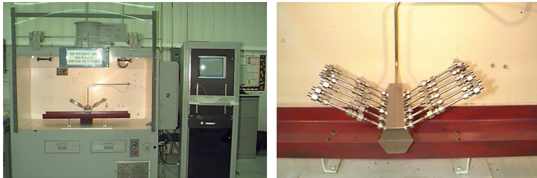
Figure 3.3.1 - 2, Hydraulic Impulse Test Stand and Fixture
