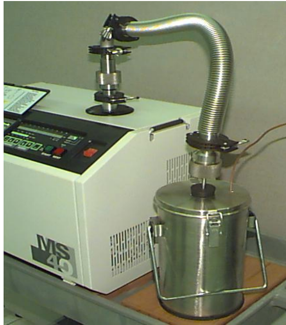
Figure 3.12.1, Low Temperature Helium Leak Test Configuration.
