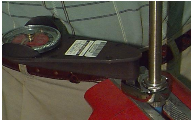
Figures 3.1.1 - 2, Initial Makeup: Torque Measurement and Fitting Assembly
