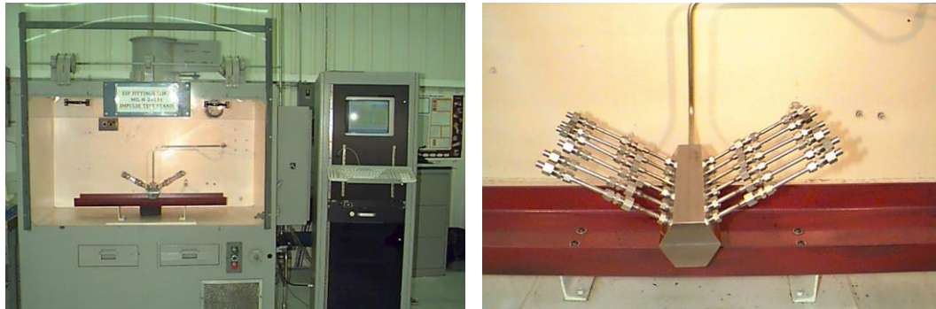
Figure 3.3.1 - 2, Hydraulic Impulse Test Stand and Fixture
