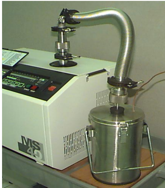
Figure 3.12.1, Low Temperature Helium Leak Test Configuration.
