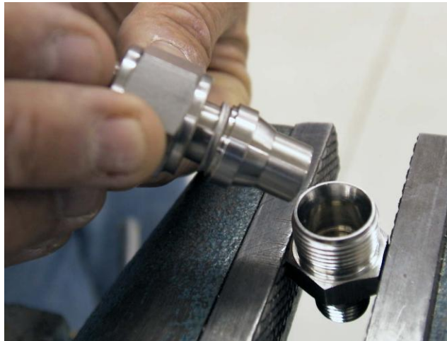
Figure 3.4.1, Repeated Remake Test (Size 8 Griplik)
